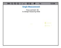
In the single measurement, long press (88) to switch continues measurement, vice versa. Aim (8) to the target, then the relevant distance will show up.
