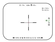
When freezing the image, you can short press MENU/REC button to adjust the X value and Y value.
