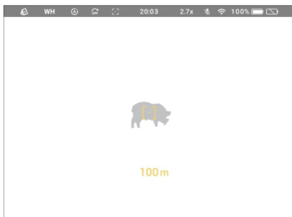
When in scan mode, aim
