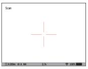
Distance to the object displays in status bar and a " + " on reticle suggests the aiming point accordingly.
