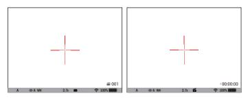
When Recording, Short press Middle Button to pause, short press Middle Button again to continue recording. Long press Left Button to exit Video and Photo function.
